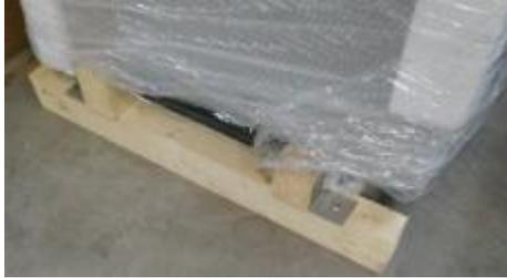
For potential handling at the installation site (positioning in the exact position), a pallet truck can be used from the side without the need for reinforcements. The pallet trolley must have sufficient length to support both legs.
