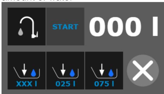
Measure the time T for how long 10 litres flowed e.g. 120 s and at the same time read the value of the filled volume V on the water control display.
