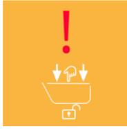
. The cover must then be pushed downwards to release the locking mechanism.
